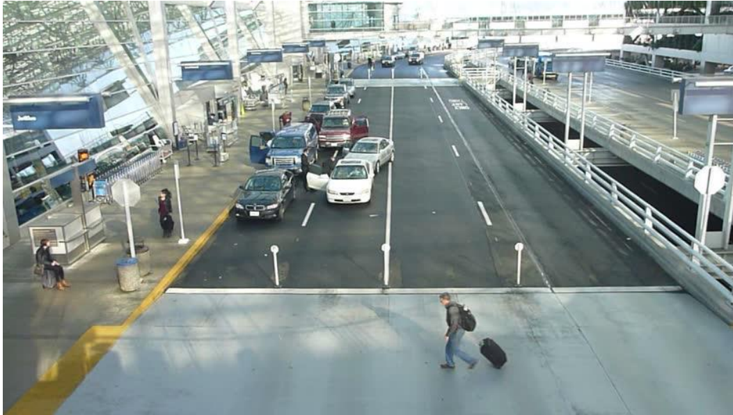
Figure 4-33: Two Lane Load/Unload Example
